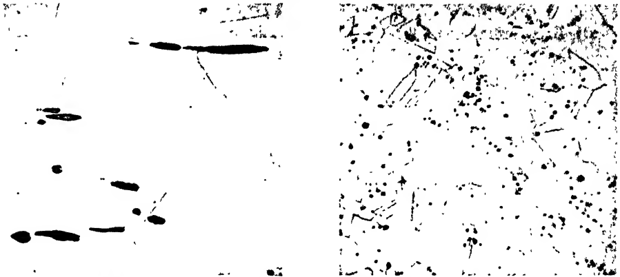
FIGURE 530. Metallographic structures of hot-rolled (left), \times 500 , and cold-worked and annealed (right), \times 200 , tough-pitch copper showing distribution of oxide. Etched with \text{NH}_4\text{OH} + \text{H}_2\text{O}_2 . (Photomicrographs courtesy (left) Research Laboratory, General Electric Company, and (right) Research Laboratory, Westinghouse Electric Corp.)
